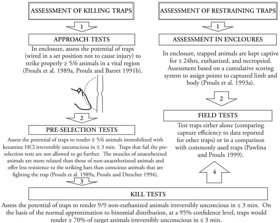
**Fig. 5.1** Sequential series of biological tests used to assess the humaneness of killing and restraining traps (after Proulx and Barrett 1991b; Proulx *et al.* 1993a).
