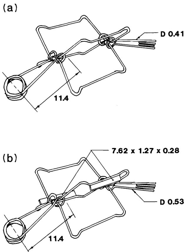
FIG. 1. Diagram of the Conibear 120 (a) and the C120 Mark IV (b). All diagram dimensions are in centimetres.
