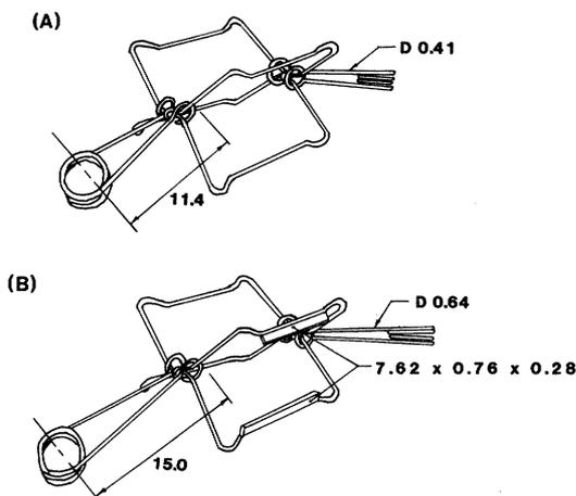
Fig. 1. Diagrams of (A) Conibear 120 and (B) C120 Magnum. Dimensions are in centimeters (D = wire diameter).
