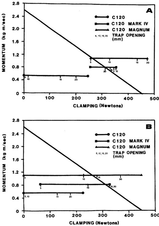
Fig. 2. Performance of Conibear 120, C120 Mark IV, and C120 Magnum on threshold graph for marten at (A) 0 firings and (B) after 10 firings.
